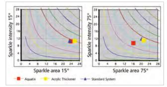
BYK-mac i measurement data correlates with a visual judgment. The sparkle area for the system with wax additive at 75° is smaller than for the two other systems. As Sparkle 75° evaluates flakes which are non-parallel oriented, this clearly shows that by using the BYK-Chemie wax additive AQUATIX® the orientation of the aluminum flakes is improved.
