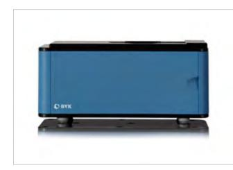
For repeatable results the product is placed into a sample drawer, which can be comfortably opened and closed. Magnets keep the drawer from sliding open. A mask is fit on top of the sample drawer to hold the micro-gloss in place and allow non-contact measurements of your products in a completely shielded compartment.
