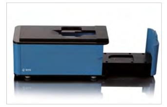
For repeatable results the product is placed into a sample drawer, which can be comfortably opened and closed. Magnets keep the drawer from sliding open. A mask is fit on top of the sample drawer to hold the BYK-mac i in place and allow non-contact measurements of your products in a completely shielded compartment.
