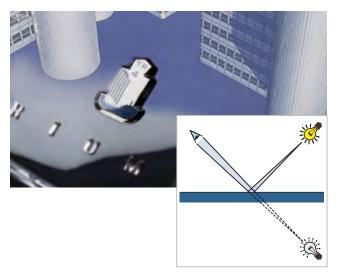
When we focus on the surface, we gain additional information about structure size and form. We see these structures as a wavy pattern of light and dark areas. This waviness is often referred to as orange peel or flow/leveling defects. Both evaluation types are individually weighted and contribute to the total appearance perception.
