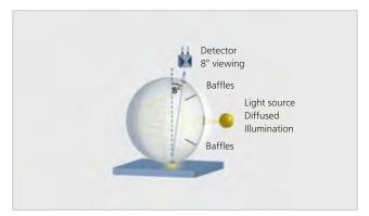
A sphere instrument may be operated under two different measurement conditions:
