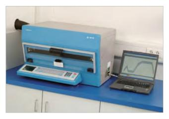
The gradient-oven helps to speed up R & D projects saving time and money. In QC testing of baked coating systems the gradientoven produces repeatable results many times faster than using traditional convection ovens.
