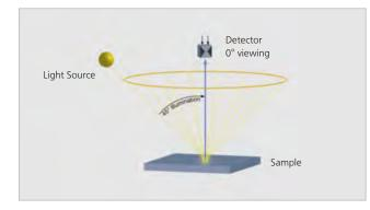
The 45/0 geometry simulates the normal condition used for color evaluation. For example, when we read a glossy magazine we position it to avoid the gloss from coming into our eye.
