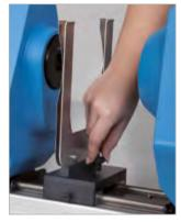
Sample holder for films and sheets. The precision guide carriage allows easy replacement of different holders.
