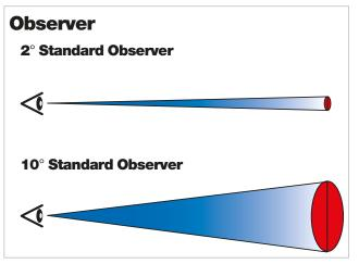
When viewing a sample, the eye integrates over a large area, which correlates best to the  $10^\circ\, observer.$
