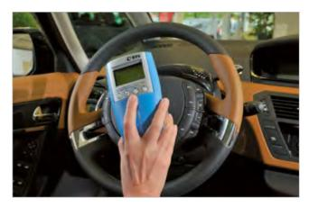
The new spectro-guide S family offers improved technical performance for  $60^{\circ}$  gloss in the low gloss range 0 - 10 GU. The excellent repeatability of  $\pm$  0.1 can be guaranteed due to a patented calibration procedure.
