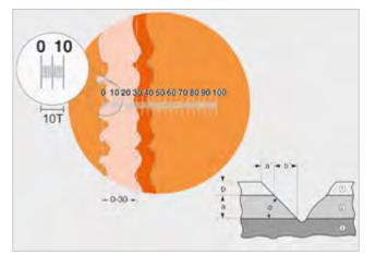
The thickness of multiple-layered coatings can be easily determined.
