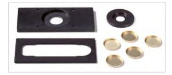
For repeatable results the product is pressed or poured into a sample cup. During sample preparation of pressed powders, it is important to always maintain the same plunger pressure as well as the same plunger tissue. It is recommended to use a fine-woven fabric to create a smooth, non-textured surface. The holder is equipped with a mask onto which the micro-gloss is placed for non-contact measurements.
