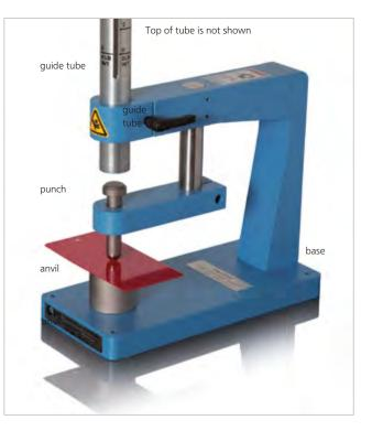
The impact force is calculated using the following equation: Falling Height x Weight = Impact Force in lbs in-lb
