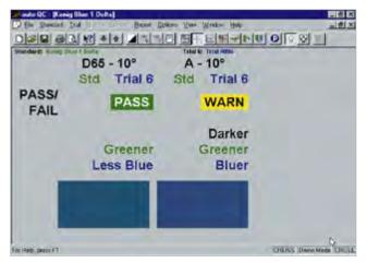
auto-QC lite automatically calculates tolerances based on measured production trials. Asymmetrical fit allows best agreement with the visual perception
