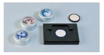
For repeatable results the product is pressed or poured into a sample cup. During sample preparation of pressed powders, it is important to always maintain the same plunger pressure as well as the same plunger tissue. It is recommended to use a fine-woven fabric to create a smooth, non-textured surface. The holder is equipped with a mask onto which the BYK-mac i is placed for non-contact measurements.
