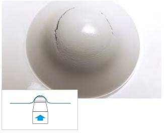
A die having a hardened and polished surface and a sample holder with a retaining ring are the heart of a cupping tester. The indenter that contracts the test panel is of hardened polished steel and forms a hemisphere of 20 mm (8 in ) diameter. The maximum cupping depth is approx. 14 mm. The test process is observed through a microscope or magnifying glass.
