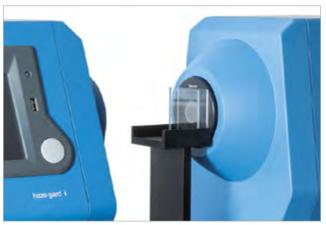
Liquids are best measured using cuvettes and the cuvette table.
