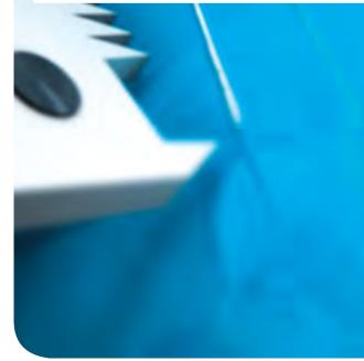
The cross-cut test is a simple and easily practicable method for evaluating the adhesion of single- or multi-coat systems.
