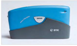
In order to obtain differences clearly, over the whole range from matte to high gloss, three measurement geometries were specified in international glossmeter standards. Each geometry is optimized for a specific gloss range.
