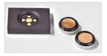
For repeatable results the product is pressed or poured into a sample cup. During sample preparation of pressed powders, it is important to always maintain the same plunger pressure as well as the same plunger tissue. It is recommended to use a fine-woven fabric to create a smooth, non-textured surface. The holder is equipped with a mask onto which the spectro-guide is placed for non-contact measurements.
