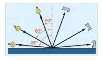
Glossmeters and their handling procedures had to be internationally specified to allow comparison of measurement values. The angle of illumination is of high influence. In order to obtain a clear differentiation over the complete measurement range from high gloss to matte, 3 different geometries, i.e. 3 different ranges, were defined:
