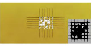
ISO Class.: 4 / ASTM Class.: 1 B The coating has flaked along the edges of the cuts in large ribbons and/or some squares have detached partly or wholly. A cross-cut area significantly greater than 35 %, but not significantly greater than 65 %, is affected.
