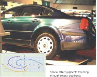
In order to fully capture the color travel of these interference pigments it is necessary to add viewing and illumination angles. To keep the whole procedure practical for industrial use with a portable spectrophotometer it was determined that an additional angle behind the gloss e.g. -15° is of benefit.
