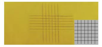
ISO Class.: 0 / ASTM Class.: 5 B The edges of the cuts are completely smooth; none of the squares of the lattice is detached.
