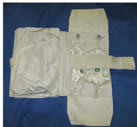
Figure 6. Water pack opened showing silver and iodine standard solutions.
